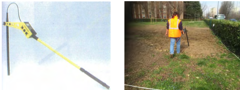
Gradiometro Foerster Ferex 4.032 DLG
