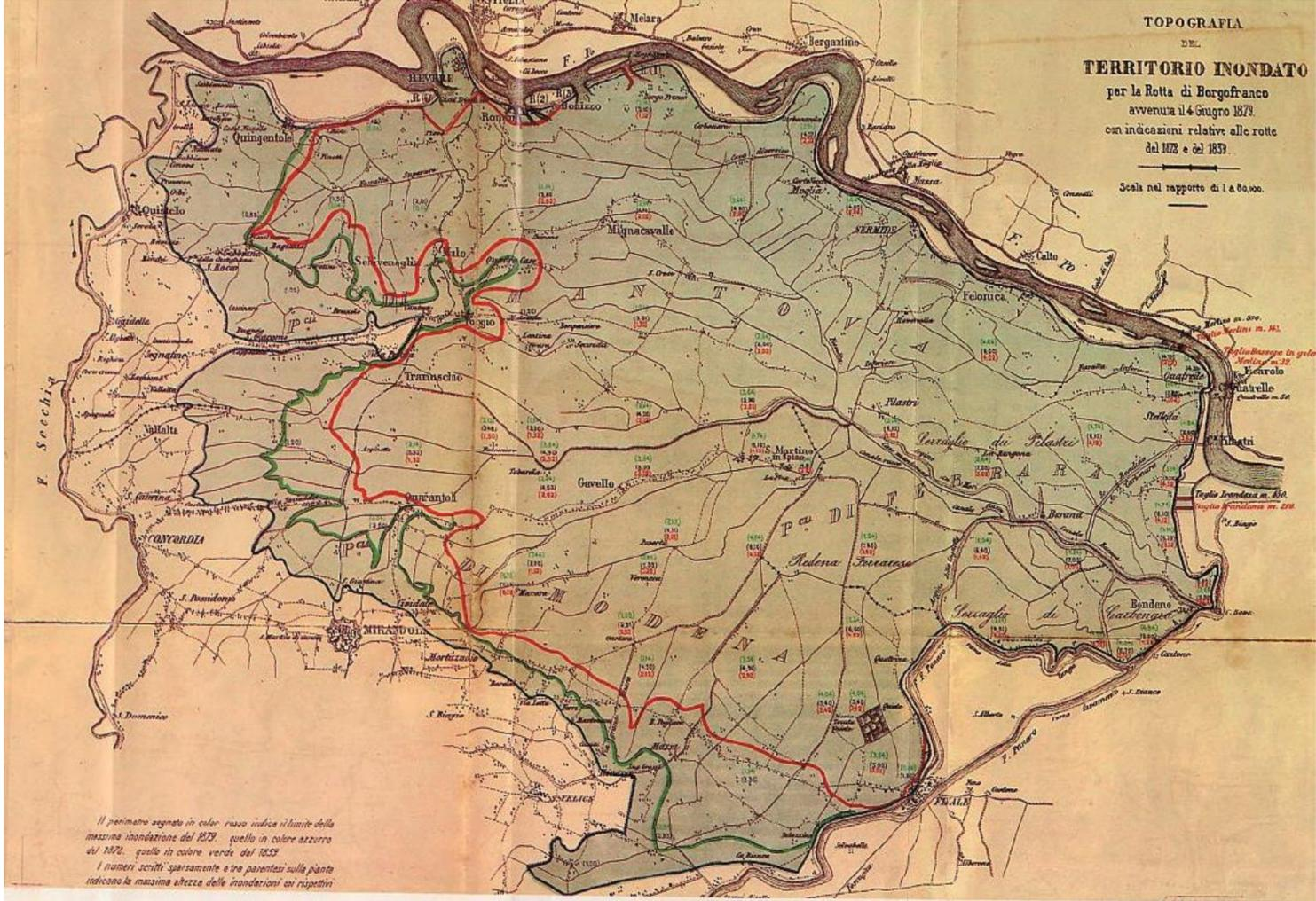
Serious levee failures occurred in 1839, 1872, 1879 in the right embankment. The inundation area, between Secchia and Panaro river, was 600 km<sup>2</sup>
